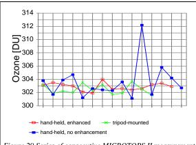
Figure 29 Series of consecutive MICROTOPS II measurements of ozone employing three different ways of sun targeting:
