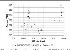
Figure 31 Comparison of Microtops II S/N 3106 with Dobson instrument #65 in Boulder CO, 08/01/96
