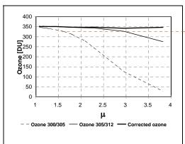
Figure 32 Measurement of ozone over wide range of air mass in Philadelphia, PA, May 31 1996.
