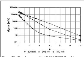
Figure 28 . Signal measured by MICROTOPS II on Mauna Loa (May 16, 1996, 271DU, clear sky)
