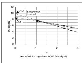
Figure 30 Illustration of the MICROTOPS II calibration procedure.
