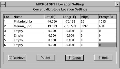
Microtops II internal location database (max. 6 locations)can be viewed and changed by selecting the **Change Instrument Locations** command on the Tools menu. Only legal values will be accepted by the Microtops. **Retrieve** will display all current locations saved in the instrument. To change the location setting, type in the new data on the appropriate line and click the SET button. All of the displayed locations will be saved to the instrument for future use.
