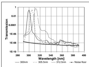
Figure 27 Spectral transmission of UV filters measured using a monochromator with 2.5nm slit width (notice bandwidth broadening) in order to detect the stray light.
