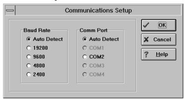
The serial port settings(com port and baud rate) can be set using the **Communications** command in the Options menu. The default settings are **Auto Detect** for baud rate as well as for com port which will automatically detect the appropriate port and baud rate for the Microtops to communicate with the PC. If the port and baud rate are not going to be changed, fixed settings can be selected instead of the auto detection process.
