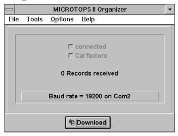
Downloading of data is accomplished by clicking the **Download** button on the bottom center of the form. Be sure that the Microtops is connected to the PC with the supplied cable and is turned on. After clicking the **Download** button, the contents of Microtops II data buffer will be copied into the DATA.DBF database located in the PC.
