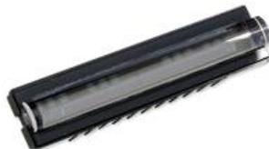
8. Detector: There are two choices of detector available for the flame. We offer a 2048-element FLAME-S (Sony ILX511B) or a 3648 element FLAME-T (Toshiba TCD1304AP) linear CCD array. These both have an effective range of 190-1100 nm. The optics split the light into its component wavelengths which fall across the different
